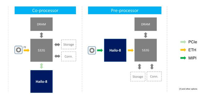
MicroSys also supports Hailo-8 Al accelerators on its NXP S32G platforms. Combining high computing performance with minimal power consumption, these accelerators are ideal for edge computing applications in vehicles.
