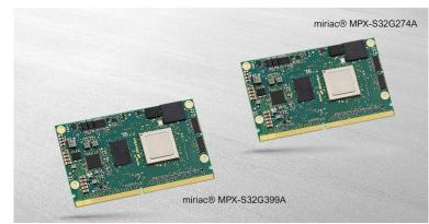
WeMOTA G2 is based on MicroSys miriac System-on-Modules with NXP S32G processors, which are predestined for use in vehicles thanks to native support of CAN, FlexRay and LIN, as well as TSN-enabled Ethernet and Ethernet T1. MicroSys currently offers two configurations, featuring either 4 Arm Cortex-A53 processors and 3 Arm Cortex-M7 processors, or 8 Arm Cortex-A53 processors and 4 Arm Cortex-M7 processors clustered as a dual lockstep pair.
