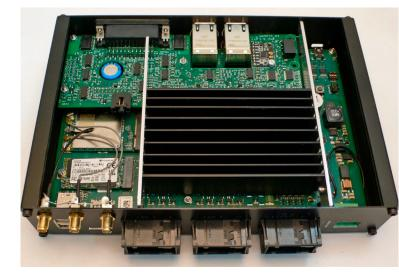
Weiß Elektronik & Software GmbH has developed a dedicated mezzanine card for analog inputs, TFT display support, GPS, acceleration and gyro sensors, and power outputs. It is mounted on the custom SBC. The WeMOTA G2 heatspreader couples directly to the housing and is milled out towards the module for an optimum fit.
