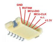
Figure 7: Module MCU Connector
