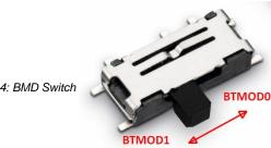
Shown positions set the corresponding BTMOD0/1 line to low. BTMOD0 controls the CPU configuration port PC9, i.e. BOOTMOD(0), while BTMOD1 is connected to the CPU configuration port PC10, i.e. BOOTMOD(1).
