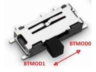
Make sure the GPU switch, located on the MPX-S32V234 module, is set properly in order to select the correct GPU supply. For more details see chapter 5.5 Switches
