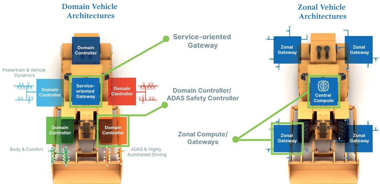
→ NXP S32G2 automotive processors power service-oriented gateways, domain controllers and ADAS safety controllers, or serve as zonal computers/gateways.
