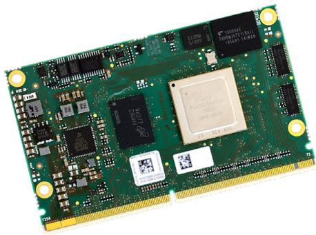
→ The MicroSys miriac® MPX-S32G274A is the world's first System-on-Module to integrate the new NXP S32G2 processor, which is specifically designed for automotive networks.
