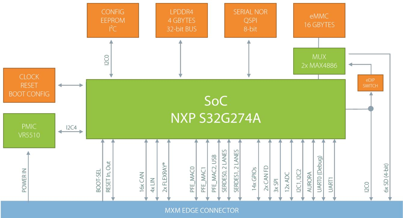
→ The MicroSys miriac® MPX-S32G274A System-on-Module provides developers with an easy-to-integrate platform that includes all I/Os of the NXP S32G274A processor, all required core components such as RAM and eMMC data storage, as well as additional interfaces.
